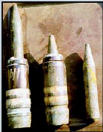
30mm DU munition: jacket and penetrator
