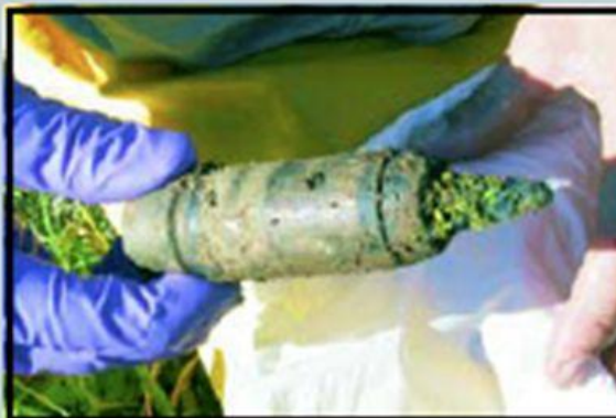
A full DU round found on a surface (penetrator already corroded)
