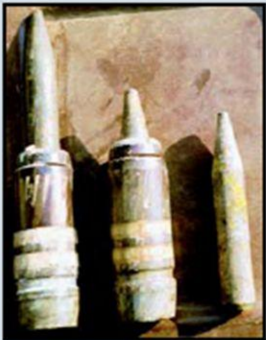
30mm DU munition: jacket and penetrator
