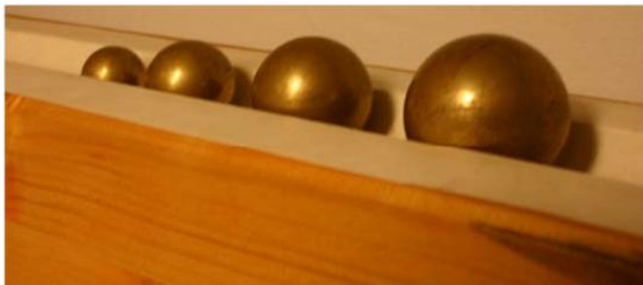
Figure 4.7 Brass balls used in the experiments placed in the reconstructed semicircle of the inclined plane
