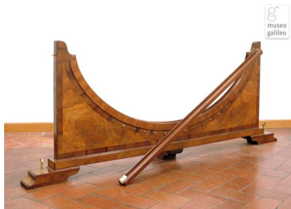
Figure 5.2 Apparatus for demonstration of brachistochronous fall
