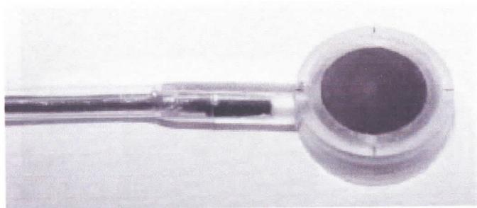
Slika 3-5 Plan paralelna komora Scanditronix Wellhofer NACP-02
