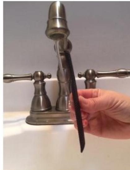
On the vertical, bring the comb toward the water (but don't touch the water) and the electricity you just generated with the plastic comb and your hair should cause the water to bend toward the comb. You may need to try it a couple of times to get it to work.
