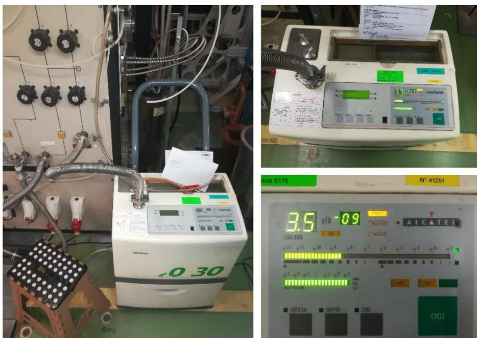
Slika 55: "Leak detector" (LD).
