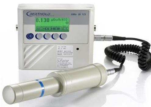
Slika 17. Berthold Technologies, UMo LB 123 dozimetar [57].
